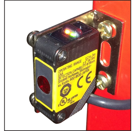
Power on & aligned
